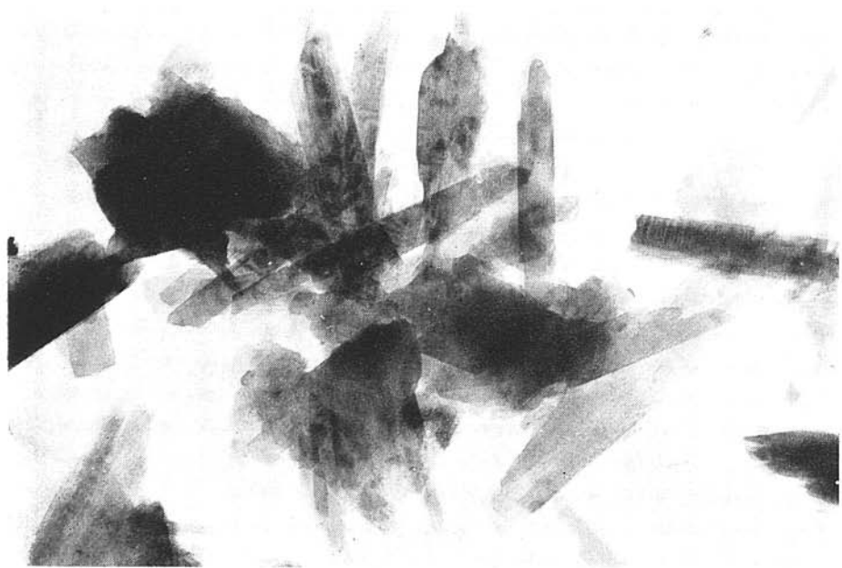
Fig. 11. Mica clay and kaolinite. Ferdinand pit, IV. horizon, sample 12. Magnif. 18 000 X.
